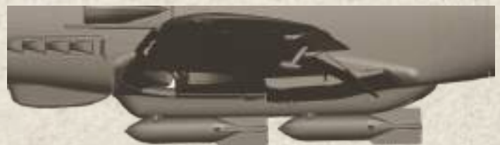
ETC 50/VIIId composite bomb rack with four 50 kg SC 50 bombs
