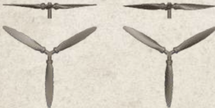
Left: VDM-9-12007.10 propeller (Bf 109 F-2 and F-4) Right: VDM 9-12087A propeller (Bf 109 F-4/Z, Bf 109 F-4 Trop)
