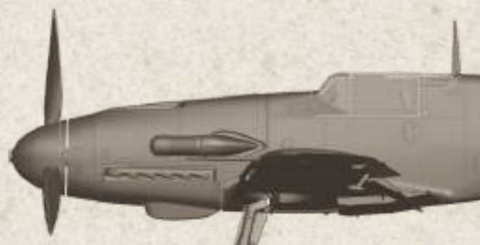
Bf 109 F-4 Trop had a larger air intake to the compressor with a dust filter. They were usually also fitted with a larger 9-6150 (Fö 870) oil cooler, and some with a VDM 9-12087A propeller with wider propeller blades.
