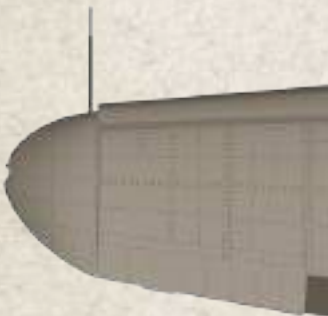
Position lights on the wing of most of the Bf 109 F-2s had no aerodynamic cover.
