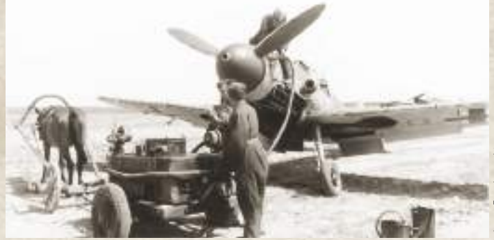
Bf 109 F-4/Z during an oil refill. The aircraft has circular wheel wells, a larger compressor intake and a VDM 9-12087A propeller with wider propeller blades.
