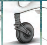
Q72391 Bf 109E Tailwheel with Strengthened Leg
